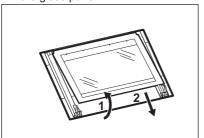
8. Clean the glass panel with water and soap. Dry the glass panel carefully. When the cleaning is completed, install the glass panel and the oven door. Do the above steps in the opposite sequence.
