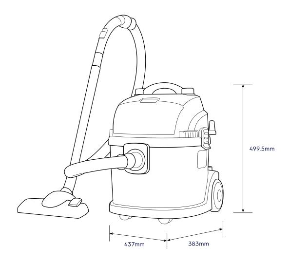
Please note! Dimensions to be used as a guide only. All customers MUST refer to the user manual supplied with the product for detailed installation instructions. © 2021 Electrolux S.E.A PTE. LTD. E\_DIM\_Z931\_Sep22
