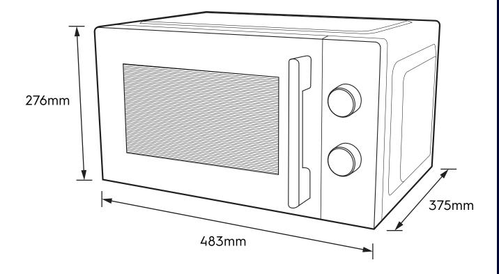
Please note! Dimensions to be used as a guide only. All customers MUST refer to the user manual supplied with the product for detailed installation instructions. © 2021 Electrolux S.E.A PTE. LTD. E\_DIM\_EMM23K22B\_VN\_Oct21
