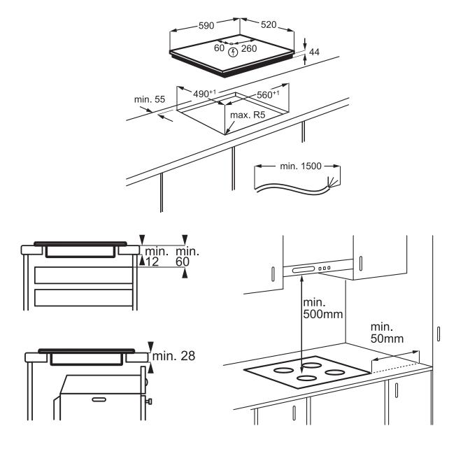
$<sup>^*</sup>$ The clearance must meet or exceed the minimum recommended for both the rangehood and cooktop. Refer to the rangehood installation manual.
