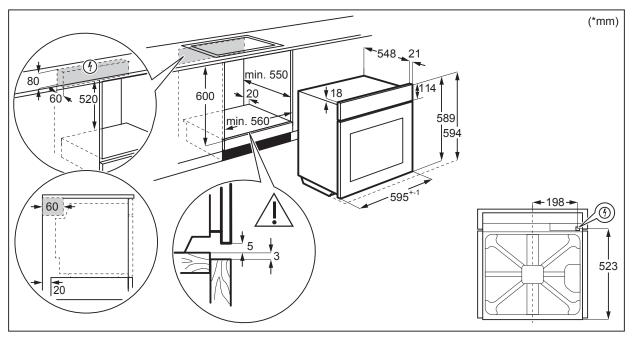
Please note! Dimensions to be used as a guide only. All customers MUST refer to the user manual supplied with the product for detailed installation instructions. KODEC75X\_Dim\_Apr21
