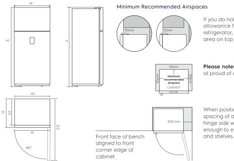
If you do not have a cupboard with allowance for air flow above the refrigerator, the recommended clearance area on top increases to 90mm.
