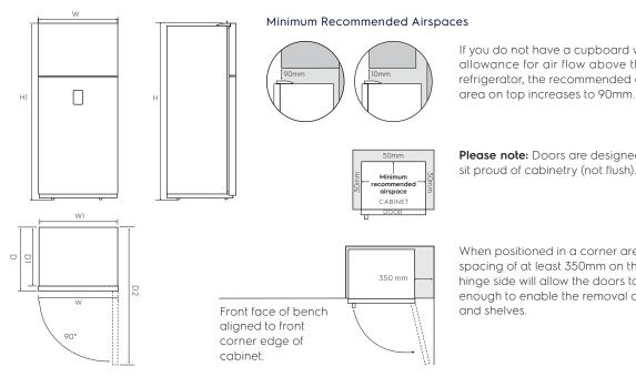
If you do not have a cupboard with allowance for air flow above the refrigerator, the recommended clearance
