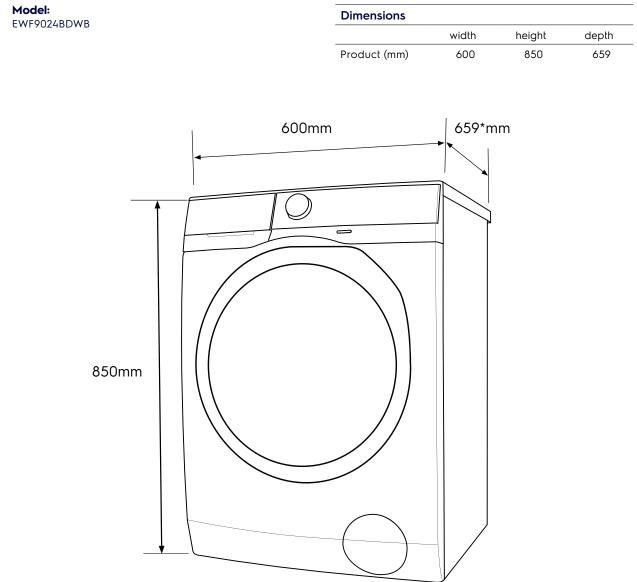
\*Add 20mm for the hose protrusion at the back.
