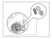
Make sure that the impeller of the pump can turn. If this does not occur, contact the service centre.
