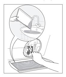
4. Push back the drainage duct and turn the filter counter-clockwise to remove it
