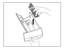
Flush it out under a tap to remove any traces of accumulated powder.
