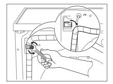
Put the end of the drain and inlet hose in a container. Let the water flow out of the hoses.
