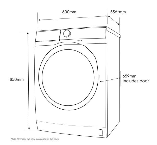
Please note! Dimensions to be used as a guide only. All customers MUST refer to the user manual supplied with the product for detailed installation instructions. © 2022 Electrolux S.E.A PTE. LTD. E\_DIM\_EWF1024D3WB\_VN\_Dec22
