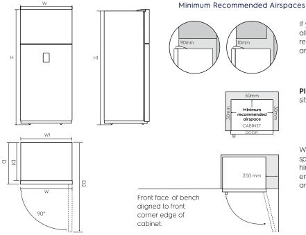
If you do not have a cupboard with allowance for air flow above the refrigerator, the recommended clearance area on top increases to 90mm.
