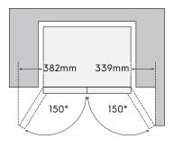
When positioned in a corner area, spacing of at least 382mm on the right hinge side and 339mm on the left hinge side will allow the doors to open enough to enable the removal of bins and shelves.
