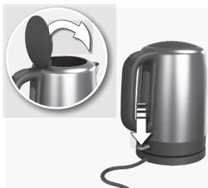
4. Close the lid (D) and make sure it snaps in correctly. Otherwise the automatic switch off function will not work reliably. **Place the jug (A) onto the base unit (I).** Press down the ON/OFF switch (H); the indicator light will illuminate and the kettle will start to heat up.
