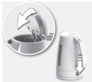
4. **Close the lid** and make sure it snaps in correctly. Otherwise the auto switch off function will not work reliably.
