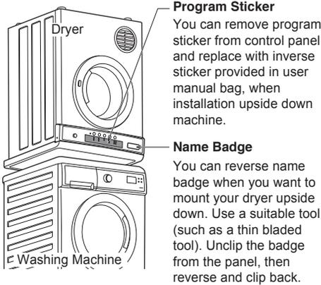
The appliance must not be installed behind a lockable door, a sliding door or a door with a hinge on the opposite side to that of the tumble dryer in such away that a full opening of the tumble dryer door is restricted.
