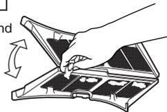
Ensure the lint filter “clicks” when replacing. It can be inserted into the pocket either way.
