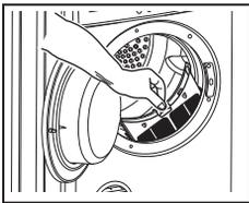
To remove the lint filter open the door and press the two pads together. Pull the lint filter out of the pocket.
