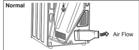
Inlet and outlet points need clear airflow to prevent overheating, so ensure there is adequate ventilation. (i.e. open window or external door.)
